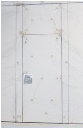
In order to ascertain the fire resistance class, a wall comprising Variflex EI 30 panels with an integrated passdoor was directly subjected to fire for longer than half an hour in a test lab.
